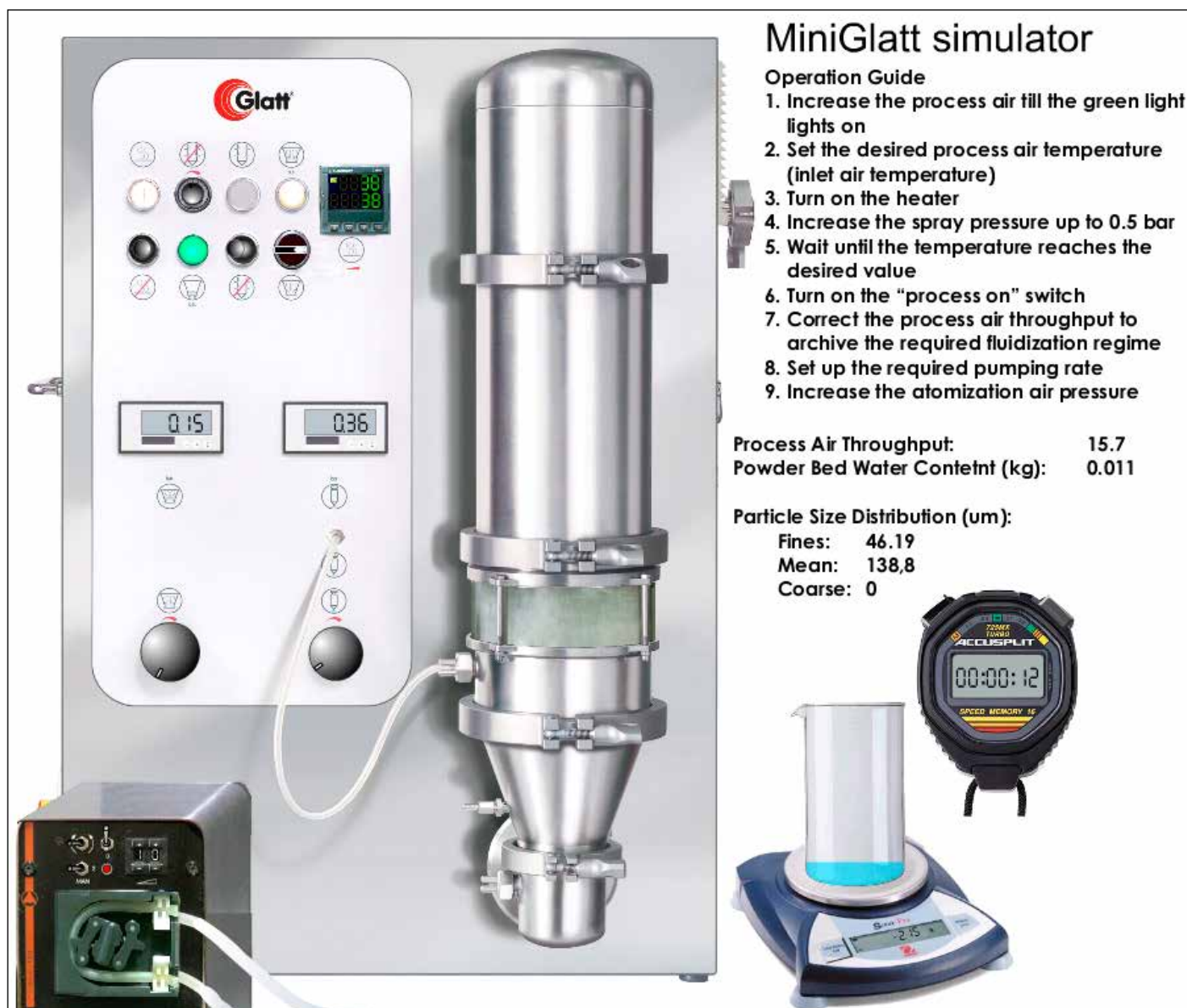
Figure 13: Screenshot of virtual equipment simulator (VES) for miniGlatt table-top processor.
