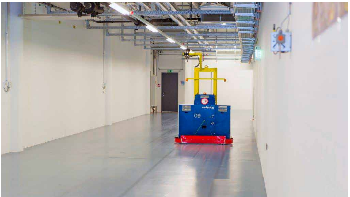
Driverless vehicles. These vehicles transport materials and waste to and from the different areas (Production and Packaging) via an underground tunnel system. Roche has 15 such vehicles in constant operation.
