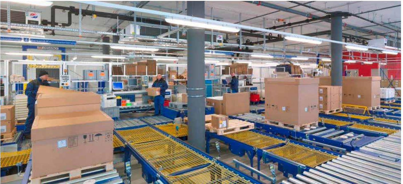
Picking zone and dispatch preparation in the refrigerated area. All the refrigerated materials needed for packaging operations and dispatch are dealt with in this area. The workstations are automatically supplied with the right material by the logistics systems.
