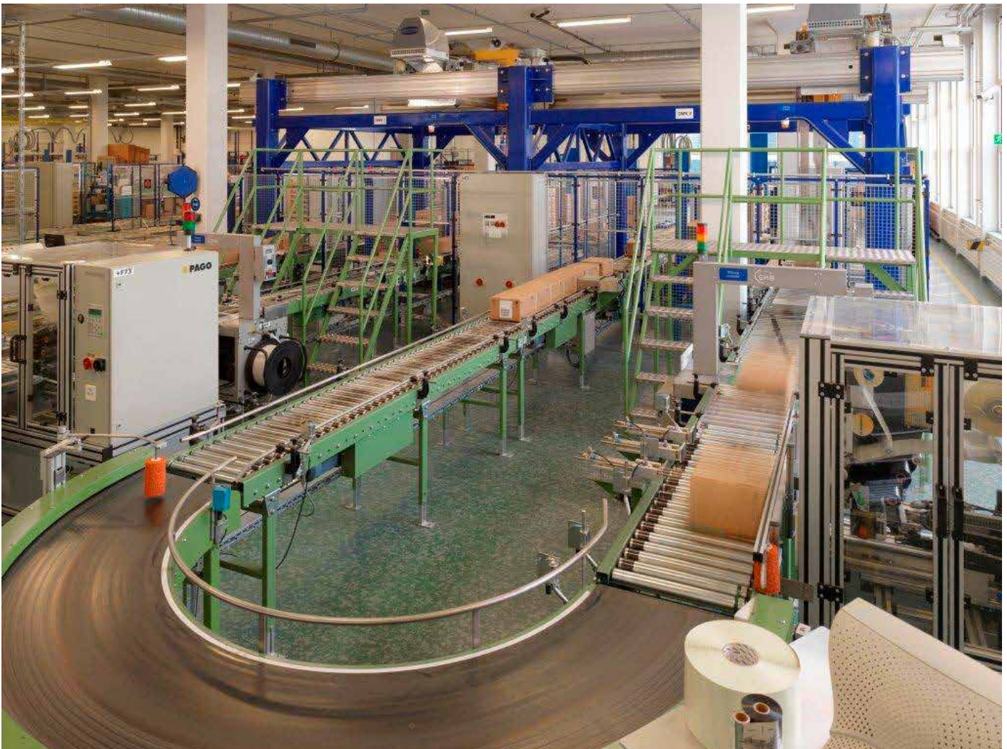
Dispatch robots (normal-temperature area). Here dispatch orders are dealt with by two robots. Each box for dispatch is automatically depalletised, strapped, weighed, labelled for dispatch and finally palletised according to the customer's requirements.
