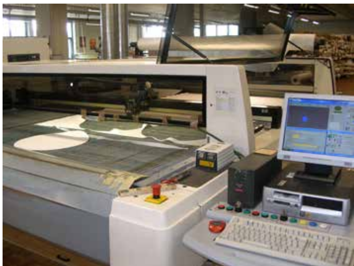
CAD controlled laser cutter. Cut width up to 248 cm.
