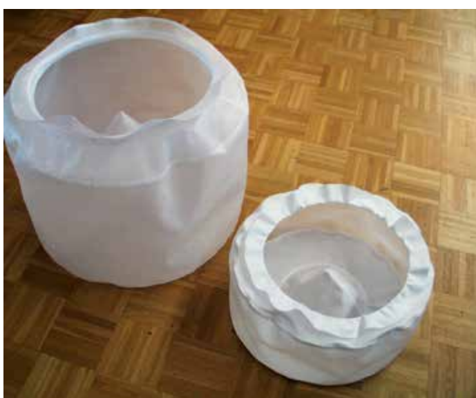
Centrifugal bags with internal taper in different sizes.
