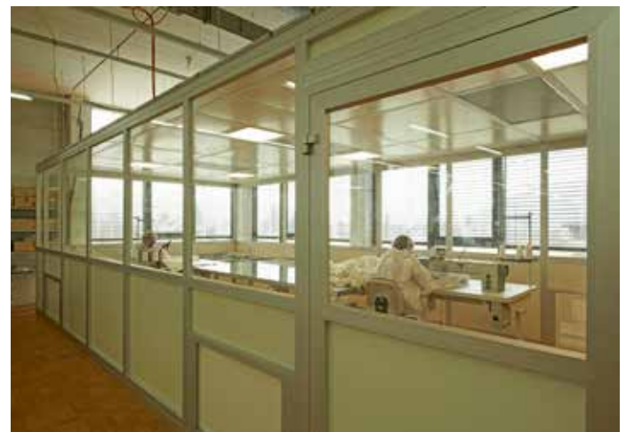
The filter production room corresponds to clean room category 7.
